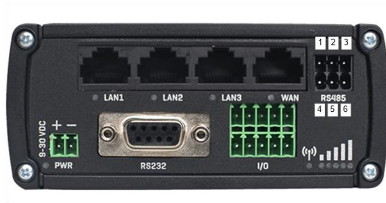
Figure 16 RUT955 – RS485 connection port
